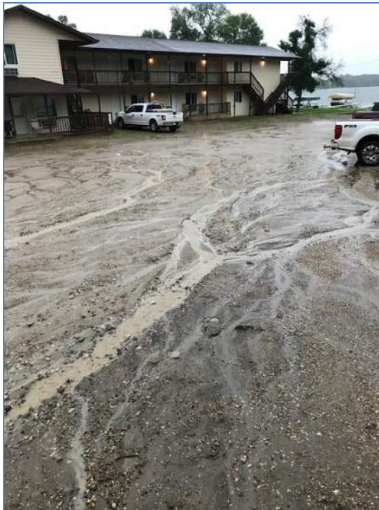
Photograph 13 is facing north from the intersection of Webster Boulevard and Huggett Lane. This is an example of where a permeable parking system would allow water to soak into the ground and runoff at a lower rate (Dan Pearson - 2019).
